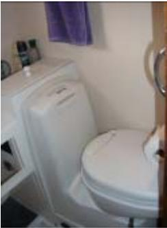
Cassette Toilet which comes in a variety of types – manual or electric flush, all have a easily removable 22 litre waste tank which you slide out and empty down any handy normal toilet. This also saves paying a boatyard to pump
